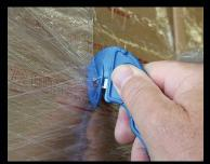
The guide angle and sharp rotating blade maintain optimum position for cutting shrink wrap for boxes and pallets. Place thumb on side grip to firmly guide your cut downward.
