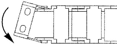
Assemble brackets to CableTrak so top surface of brackets are in same plane as outer curved surface of CableTrak
