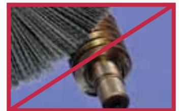
INCORRECT Point of Contact
