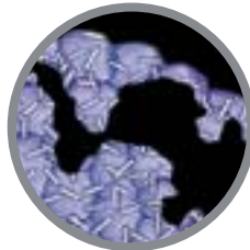
3M™ Ceramic Abrasive Grains with Platelets
