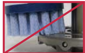
INCORRECT Point of Contact
