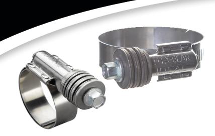
Flex-Gear® Constant Tension Clamps use a 300SS Belleville spring design which maintains constant tension on the connection, eliminating leak paths, making them an excellent choice for fluctuationg temperature applications and thermal compensation. The Flex-Gear® clamp is designed with a lined band, protecting the hose from shearing, extruding, or imprinting when the clamp is tightened.
