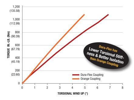
The Dura-Flex elastomer coupling has been proven to optimize torque transmission, while minimizing parallel, angular, and axial stiffness.
