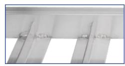
Single-Deep Shelving units are constructed of 2¼" x 1¼" x .100" thick T-shaped laterals, spaced 1¾" apart.
