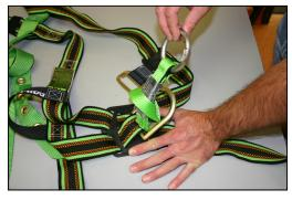
Pull O-ring extension taut to secure a snug fit.
