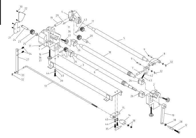
Figure 2 – Repair Parts Illustration for 36" slip roll (13W882) and 50" slip roll (13W883)
