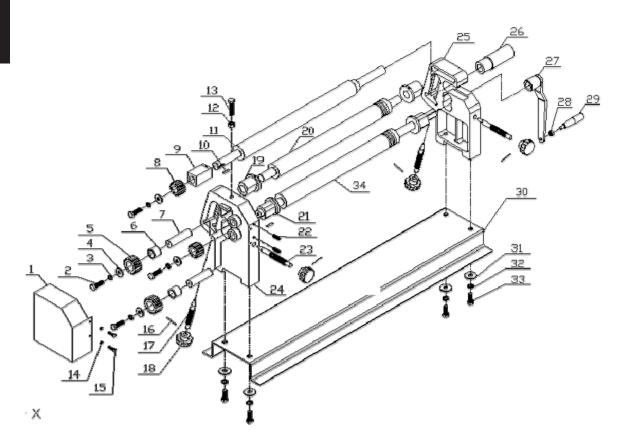
Figure 1 – Repair Parts Illustration for 24" slip roll 13W881
