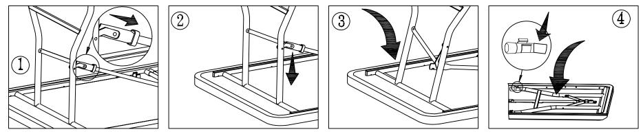
release the safety lock as shown before to fold legs.
