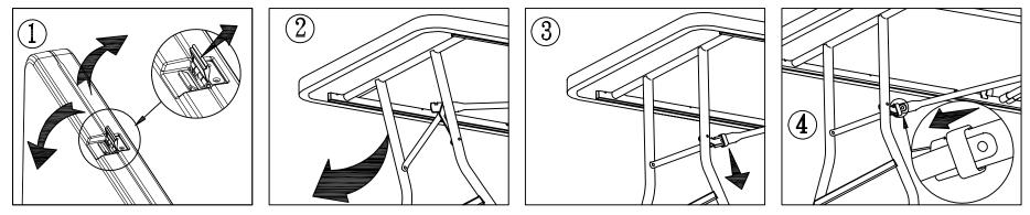
make sure that safety lock is in locked position as shown after opening legs.
