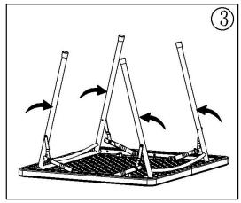
release the safety lock as shown before to fold legs.
