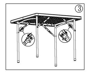
make sure that safety lock is in locked position as shown after opening legs.
