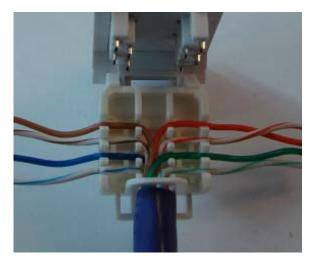
**Step 2.** Open the lid of the keystone and insert the wires through the loop at the end. Untwist and splay out the wires and sort them through the appropriate slots on the lid. Follow the color coding diagram on the side of the lid for the proper wiring standard you wish to use.
