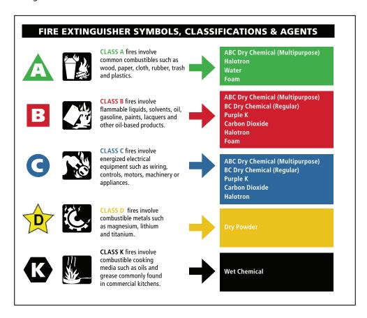
Note: Although ABC and BC Dry Chemical extinguishers can control fires involving electronic equipment, the National Fire Protection Association Standard for portable extinguishers (NFPA-10) advises against dry chemical extinguishers for fires involving delicate electronic equipment due to potential damage and clean up issues presented with agent residues.
