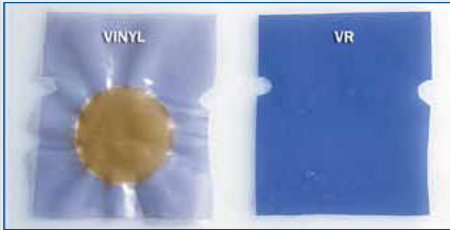
Sulfuric acid exposure test show the exceptional properties of VR™ as compared to vinyl.
