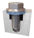
For slotted holes or on soft material, use a flanged nut/ bolt in combination with Nord-Lock "sp" (enlarged outer diameter) washers.
