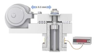
The Junker vibration test to DIN 65151 is an excellent method for testing and comparing the security of bolted joints. During the test, the joint is subjected to transverse movements while the tension is being continuously measured by a load cell.
