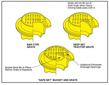
Selection of Top Material—(Unfinished Areas)—Drains located in heavy traffic areas should be specified with heavy duty cast iron grates. In areas where shock loads are anticipated, a ductile iron grate should be specified in lieu of the cast iron grate. Cast iron is acceptable for most unfinished areas such as warehouses, loading docks, boiler rooms and similar areas.
