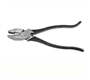
Klein Tools Ironworker's Pliers have aggressive teeth for a strong grip when twisting, snipping and pulling soft annealed rebar tire wire. The knurled jaws aid in easy twisting and turning. These pliers feature a hook-bend in the handle for added grip and leverage. Unique handle tempering helps absorb the "snap" when cutting wire.
