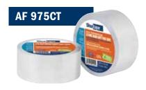
Cold temperature aluminum foil tape for use in temperatures ranging from -20 F to 260 F when joining and sealing aluminum-backed or fibrous insulation and metal ductwork, as well as when repairing metal and sheet metal. AF 975CT is linered, designed with an acrylic adhesive, tested in accordance with UL 723 and delivers an airtight seal every time.
