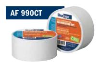
All Service Jacket (ASJ) tape for use in cold and dual temperature systems to seal, seam and join scrim-reinforced pipe and duct insulation. AF 990CT is linered and offers an acrylic adhesive, performs in temperatures ranging from -20 F to 260 F and is tested in accordance with UL 723.
