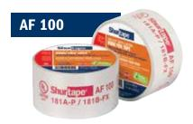
UL 181 A-P/B-FX Listed aluminum foil HVAC tape for joining and sealing joints, connections and seams on rigid fiberglass ductboard and flexible air duct. A tape that "does it all," AF 100 is engineered to form airtight bonds on joints and seams in application temperatures ranging from -20 F to 260 F and in humid conditions.
