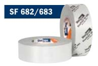
ShurFLEX\* HVAC professional grade metalized cloth duct tape designed for airtight and moisture-free seaming, connecting, splicing, patching and sealing of sheet metal and flex duct, rigid duct boards, air vents, insulation, fibrous filter banks and pollution collection systems. For superior performance, SF 682/683 is easy to use, hand tearable and designed in color and appearance to match sheet metal, flex duct and ductboard.
