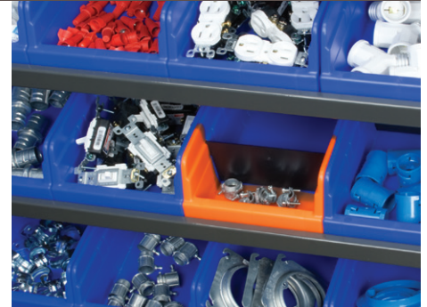
A complete Kanban system in a single bin The orange/red trigger side indicates when supplies need to be replenished.
